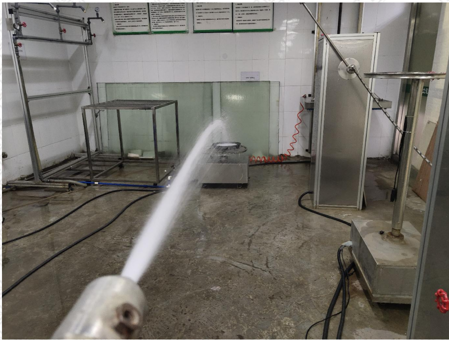
Photo 4: IPX6 test of model GL-UFO200-L
