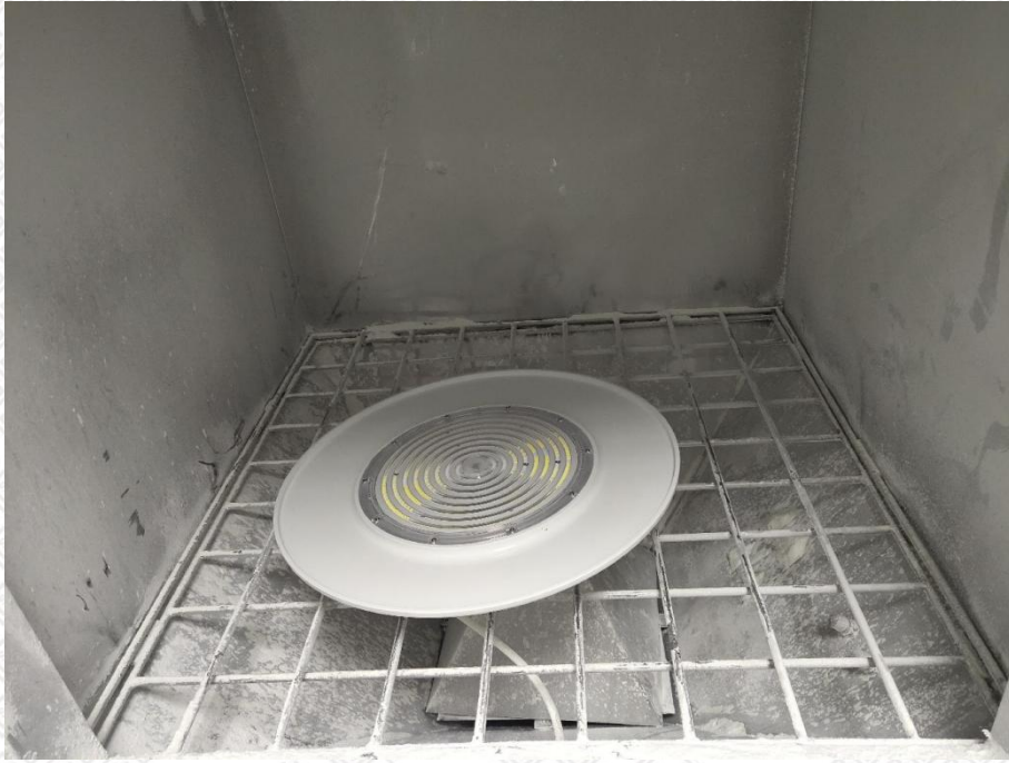
Photo 15: IP6X test of model GL-UFO200-V
