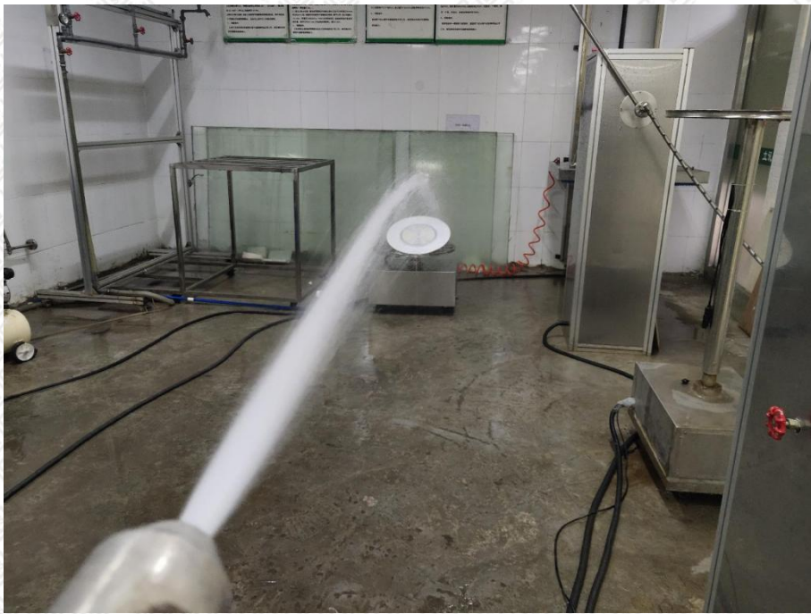
Photo 16: IPX6 test of model GL-UFO200-V
