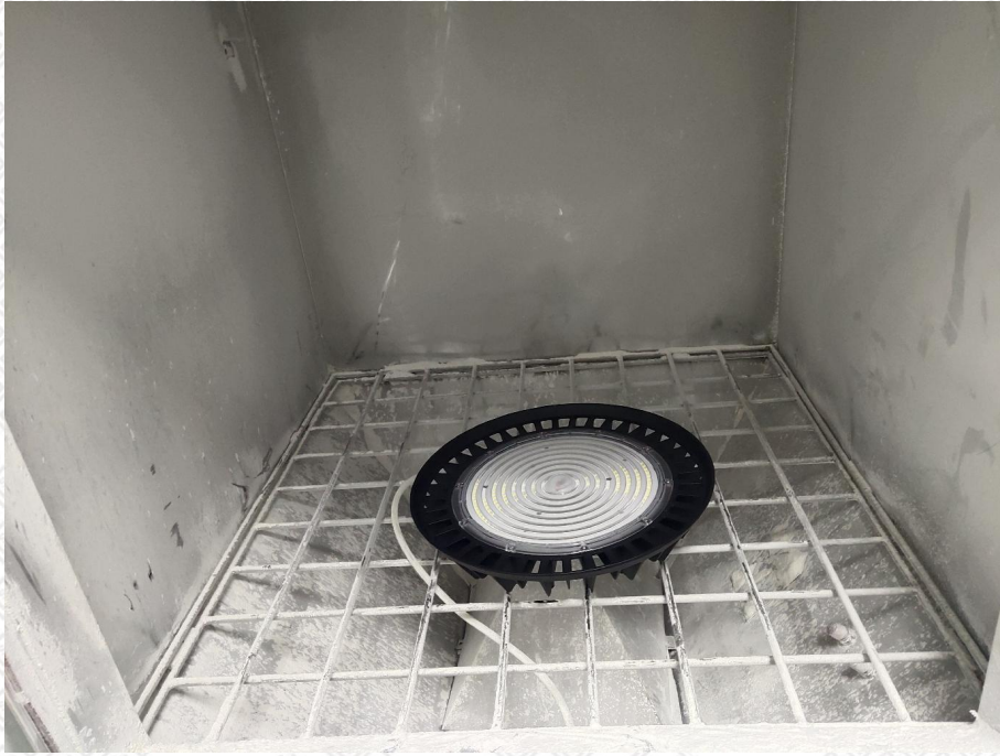
Photo 3: IP6X test of model GL-UFO200-L
