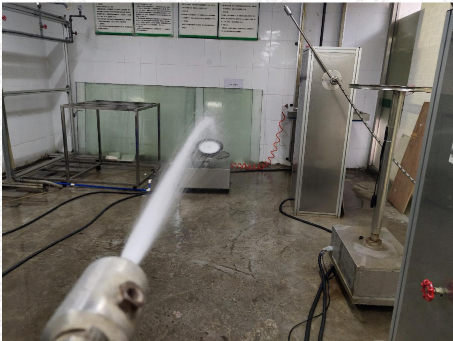
Photo 10: IPX6 test of model GL-UFO200-V
