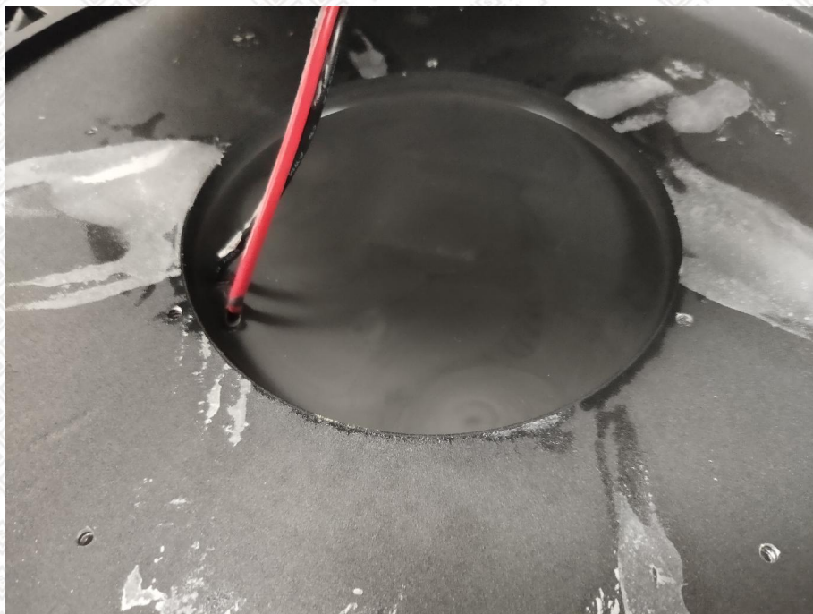
Photo 6: Test result after IP6X and IPX5 test for model GL-UFO200-L
