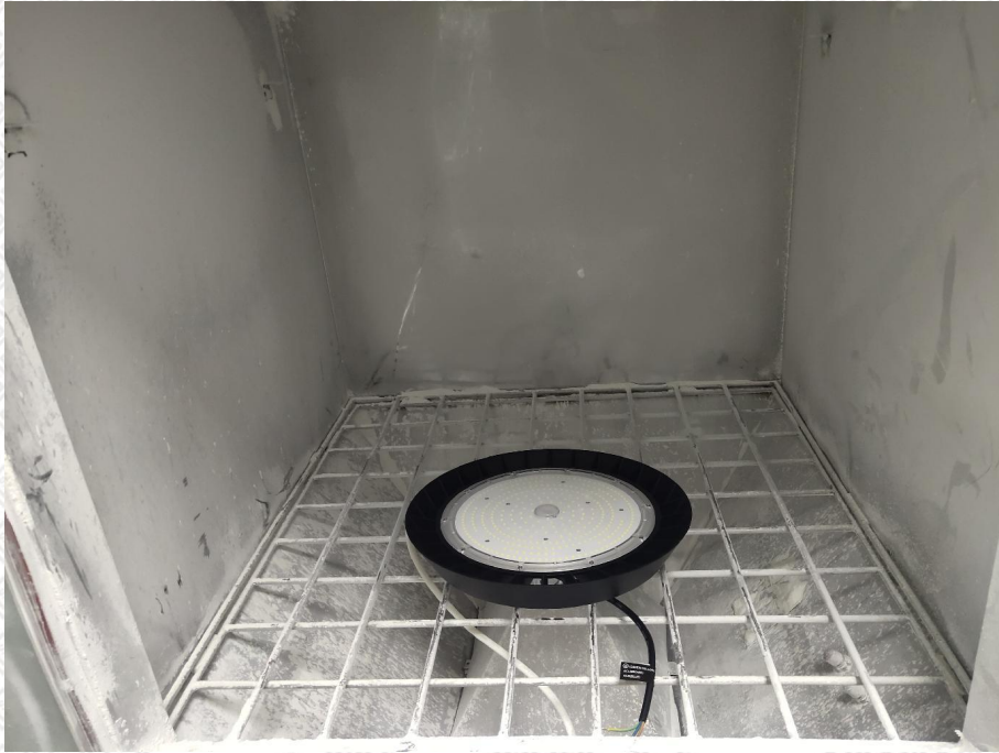
Photo 9: IP6X test of model GL-UFO200-V
